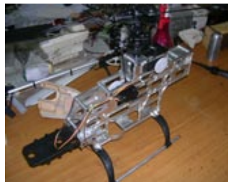
Carved from a solid billet of aluminum by a Swiss CNC mill, this glimpse of a prototype is sure to whet the appetite of electric enthusiasts. But before you're carried away imagining an aluminum side frame model, you should realize these aluminum frames mass about twice that of the final molded-plastic parts. Also, sharp-eyed readers will see another prototype just behind this one. We're always thinking of new models but the exciting thought to take from this photo is the observation that other than the frames, all the Tiger 50 components are reused. If this makes it to market, wouldn't it be neat if it were offered just as an economical electric side frame conversion kit? Tell us what you think!
