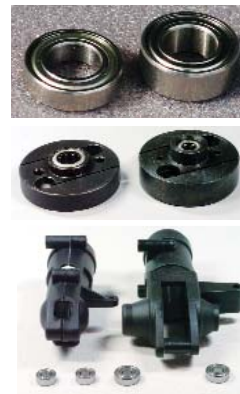
Top: The Pantera P6 main shaft bearing on the right compared to a competitive .50-size heli. Center: No one can fault Audacity for making a light-duty heli. Here you can see the P6's clutch on the right as compared to a competitive 600-size nitro heli. Above: The Pantera P6's tail case and bearings on the right compared to a competitive .50-size heli.
