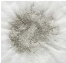
After 4 flights we cleaned the air filter through a coffee filter and this is the debris that would have otherwise been sucked into your engine.
