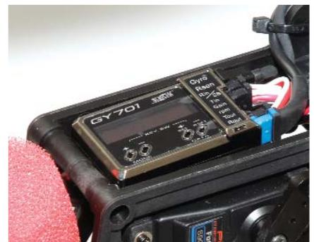
**The Futaba GY701 installs perfectly in between the frames on top of the front cyclic servo. This makes access to the unit much easier when you need to make adjustments.**
