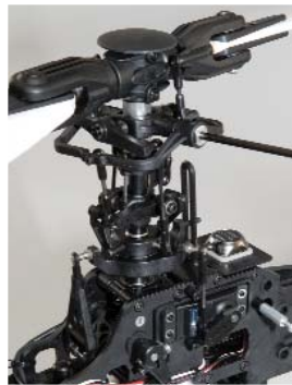
This is one heavy-duty main head, especially for a .50-size heli. Audacity touts it as a "programmable head" because there are multiple adjustments that can be made to cater the P6 to your particular flying style; from very docile to extreme 3D.
