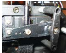
Audacity's options Servo Output Shaft Stabilizer can be added to each servo. They provide additional support and take the brunt of the force off the rubber mounts and focus it onto the center pivot point of the servo. These are a must for heavy 3D flight.
