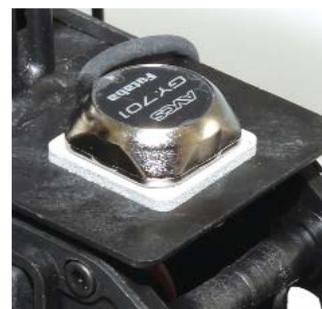
**The gyro tray is located just behind the anti-rotation arm keeping it very close to the main shaft's centerline.**
