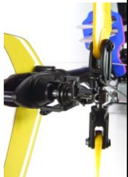
The pitch slider has two bearings for reliable operation, and it’s guided by forked bellcrank that uses dual pins.
