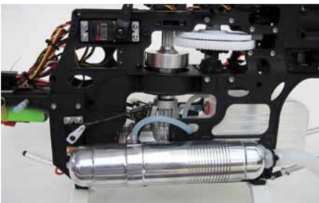
With the Hobbico LiFeSource battery mounted below the tray, the Hitec Optima 9 receiver has plenty of room on the front of the Pantera P6. Note the heat sinks on the Hitec HS-7945TH servo and the beautiful Audacity ProMuffler V2.
