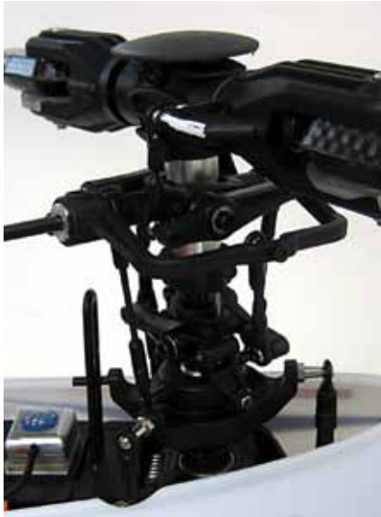
The CCPM swashplate has direct servo control to give the P6 a “locked in” feel, and I really like the molded flybar cradle and the gyro mounting plate. Note the tiny Futaba GY-520 gyro and the white mark used to note the master blade grip.
