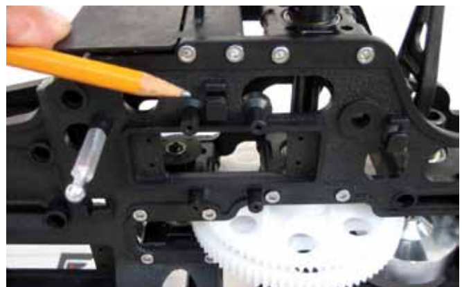
See the text for all the design features built into the fiber-reinforced side frames. Here I’m pointing to a tab used to secure the servo wires. Note the molded servo mount, the gyro mounting tray and the Delrin gears.
