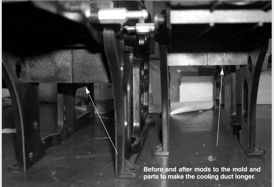
Before and after mods to the mold and parts to make the cooling duct longer.
