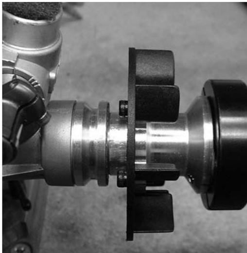
**Fan/clutch assembly on engine with prop drive.**
