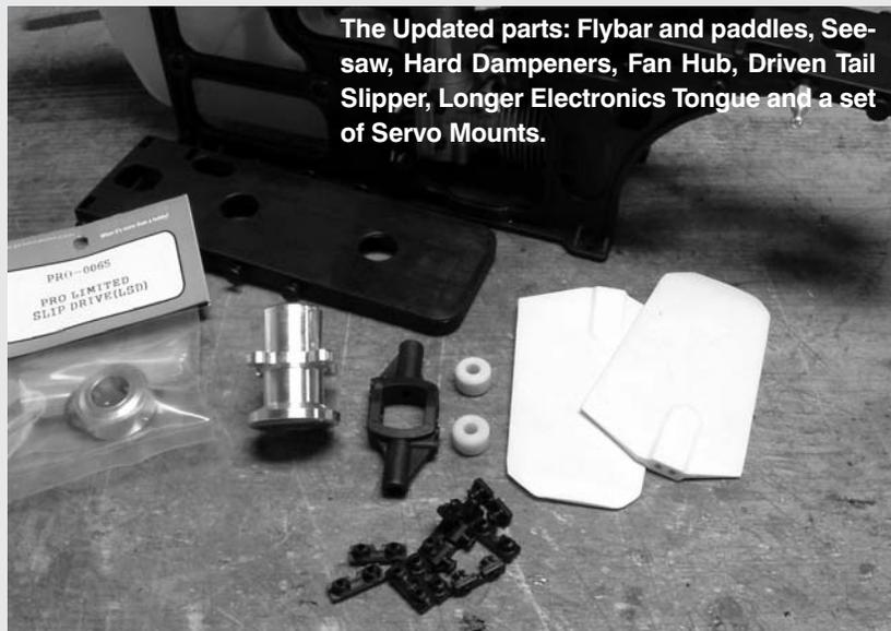
The Updated parts: Flybar and paddles, Seesaw, Hard Dampeners, Fan Hub, Driven Tail Slipper, Longer Electronics Tongue and a set of Servo Mounts.
