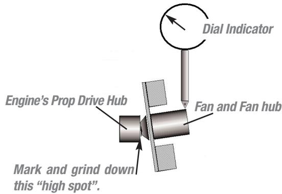
Using a dial-indicator to get the fan hub run-out true
