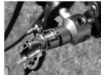
of confidence, I swapped out the stock tail hub assembly with one off another machine (a Venture 50) so I could keep flying until new parts came in. New bearings solved the problem.
