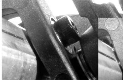
**This is more irritating that critical but this seesaw bolt contacts the mixer arm when the arm is in the hole closest to the pivot.**
