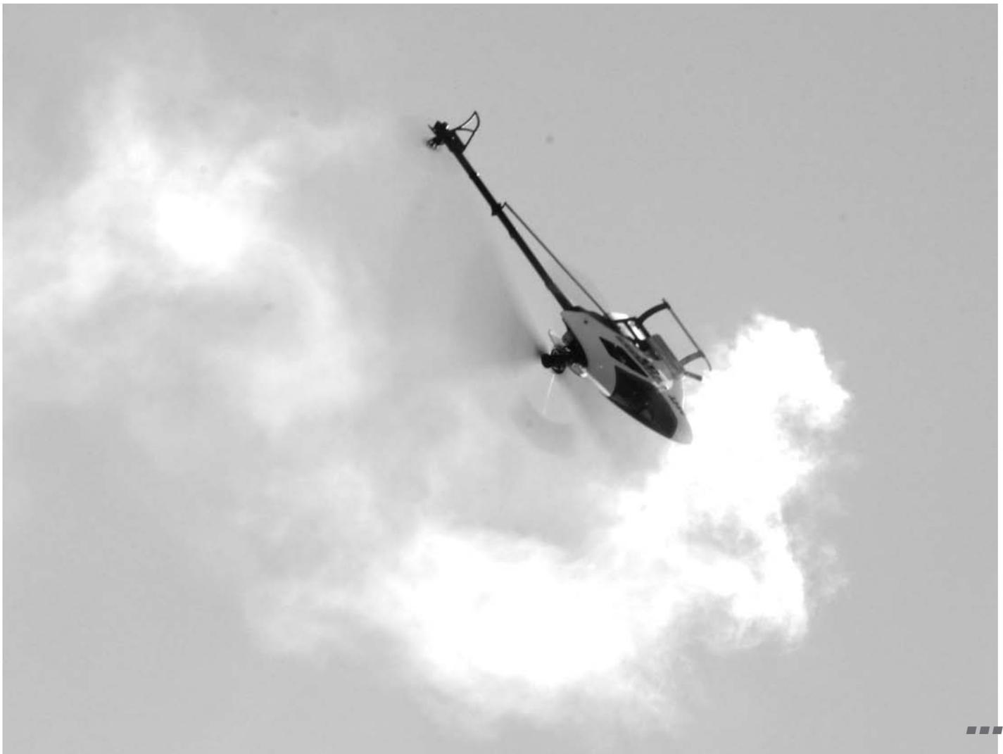
**Forward facing muffler keeps machine cleaner but does not affect performance. and also helps out the CG placement. Skeletonized vertical fin is from Mr Carbon and was borrowed from the Scedu EVO. Tiger has very good tail power due to 5.2:1 ratio. For comparison: Venture 50 is 5.18:1, Scedu Evo 50, 4.65:1 and Raptor 50, 4.56:1. The MHT Tiger came in at 8.0 lbs with 1/2 tank of fuel and header tank.**
