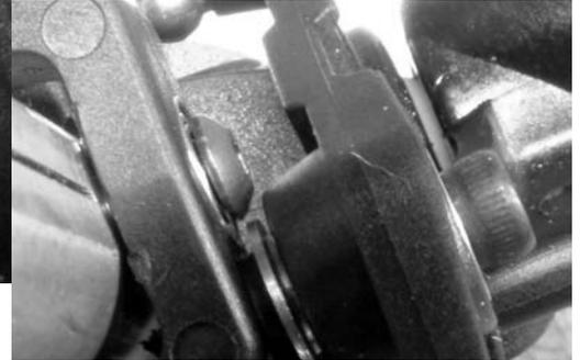
**Here is the solution the seesaw bolt hitting the mixer arm ... a pan head replacement from the Ace Hardware Store.**
