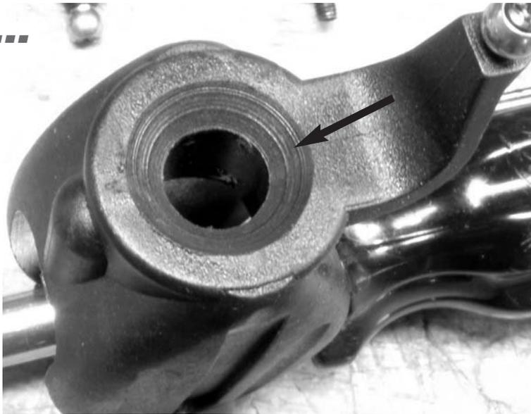
I opened up the main blade grip with a countersink to allow more room for the yellow dampeners to squeeze around and clear the grips when the head gets "active". Otherwise, the grips have been working great with absolutely no plastic "creep" affecting the vital bearing fit.
