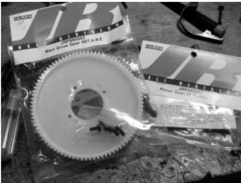
Here's the hot setup for a better gear ratio for the Tiger. This will allow the Hyper50 to do it's best. Due to the long reach the the typical Governor installation needs to get to the fan itself, I relied on old school pitch curve setup to get my machine sweet. This gear set really made that an easy task without the OS going ballistic in fast descents or when the disk unloaded in 3D.
