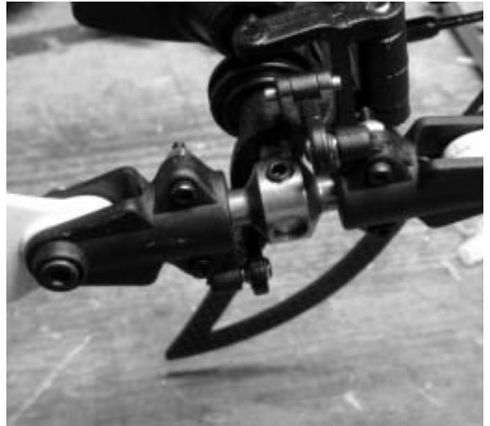
*Todd Dudek has developed these dampeners for the Scedu Evo 50. The concept is that they are soft around center but the spindle can essentially bottom out, hence tighten up, when asked to do 3D aerobatics. They are working well in the MHT Evo so far! See Finally .... for more info on Todd's products.*
