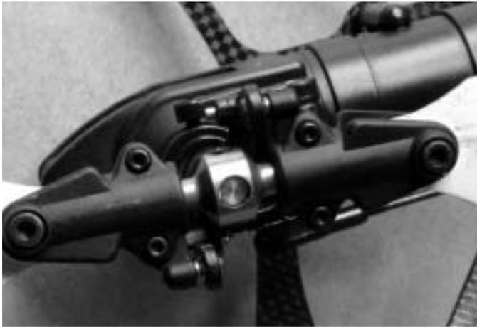
*And here are a couple of shots of the Tail Hub assembly from JR fitted to the Tiger. I had a few stock Tiger bearing failures and wanted to make sure that this system was solid.*
