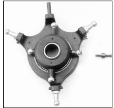
**The swashplate ball spacers. One is installed on the right ball with the other spacer and long bolt next to it. Note the difference between the stock configuration on the left and the ball that has been spaced out on the right.**
