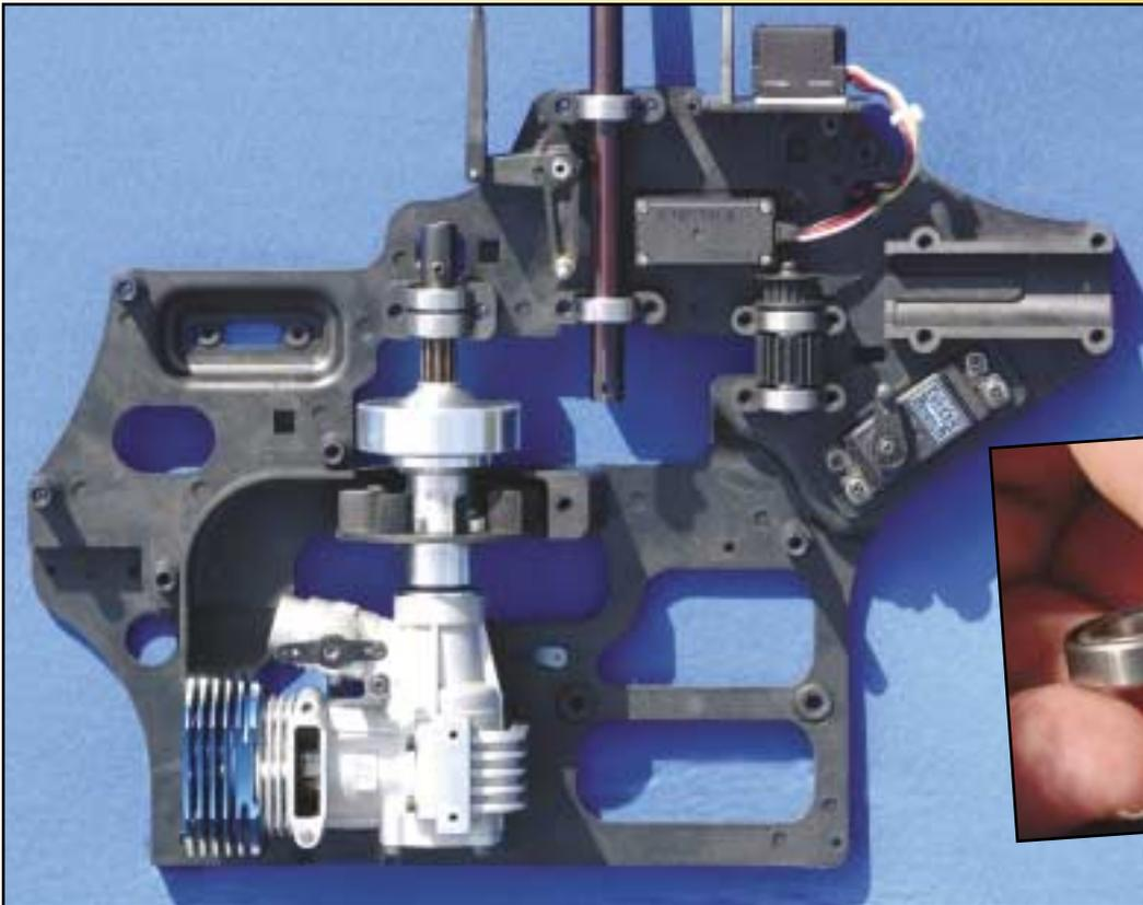
Beefy side frame features thick 7 mm bearings, spreading the flight loads to prevent the seats from prematurely wearing and exhibiting excess play. Also note how installing the servos directly in the side frames means they're protected in a crash.
