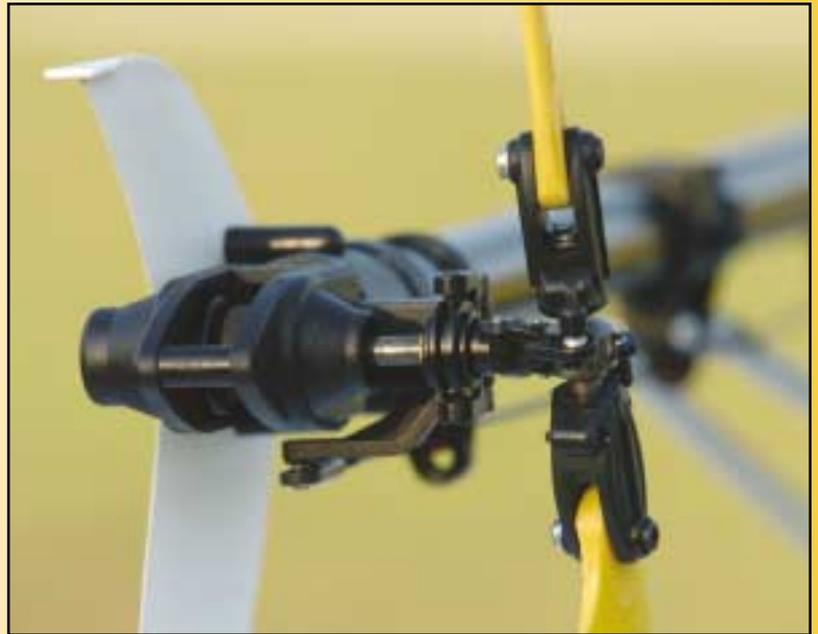
Servicing the tail rotor gearbox is quick and easy because three screws grants ready access for maintenance or repair without removing the belt, the boom, or the gear box itself - sweet!
