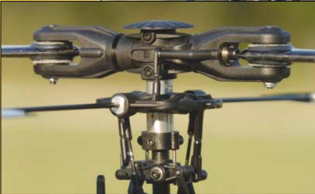
Equipped with an aluminum head block as standard, this feature is usually found on more expensive helicopters, or as an upgrade in the 50-class. This ensures the Tiger 50 has the right stuff for aggressive 3D flight straight out of the box.
