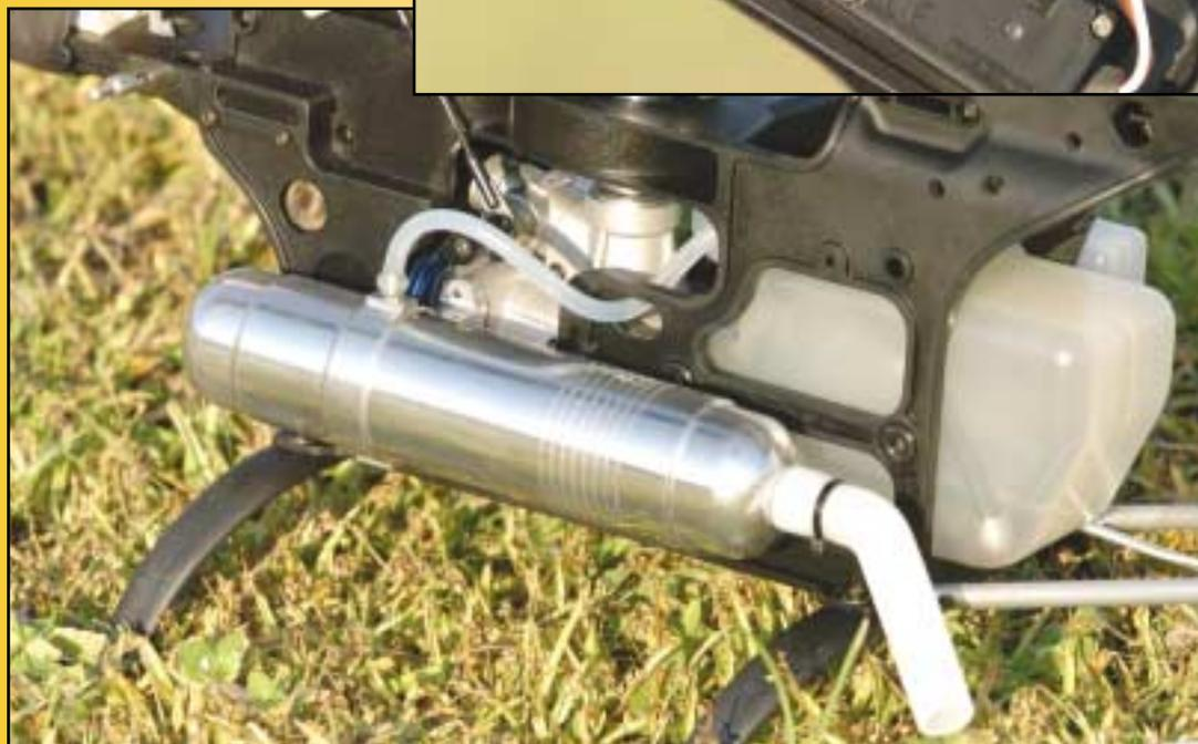
Perfectly suited to the OS Max 50SX Hyper, the ProMuffler isn't merely a re-labeled 46-class muffler but a true 50-class exhaust system. Featuring a nice throaty rasp, it lets the Hyper sing its song, i.e. deliver the goods, without excessive noise.
