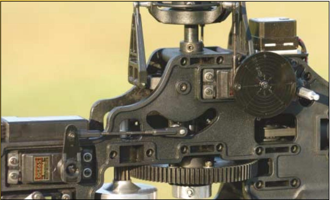
Above: Sophisticated yet simple, the Tiger 50 features CCPM. With only 1 linkage and 3 pushrods between the servos and the swashplate, the result is less slop than conventional mixing systems due to fewer pushrods and linkages to wear, or repairs following an accident. Note the use of Allen-head bolts throughout the construction of the Tiger 50 instead of cheesy Phillips-head screws.
