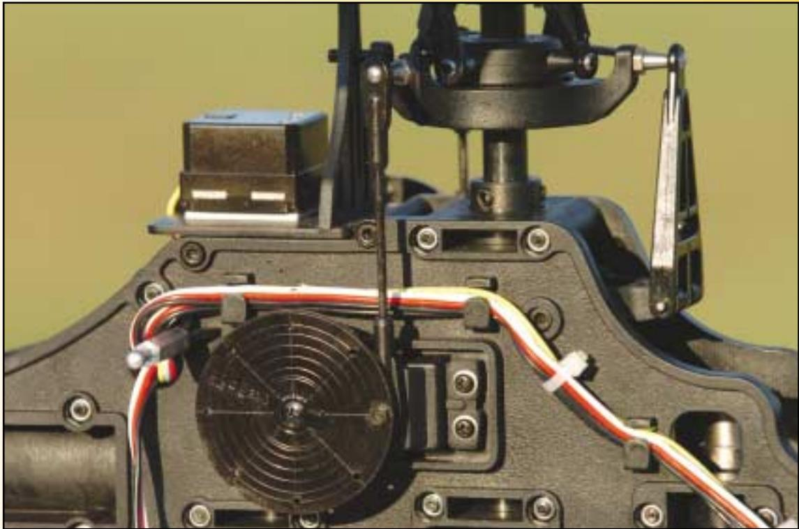
Nicely thought out guides for the servo and gyro wires means an organized wiring harness isn't an afterthought, but a feature that's designed into the Tiger 50.
