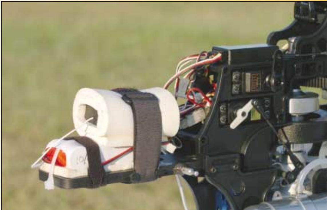
Note the boss molded in the recess of the tail boom clamp area in the aft part of the side frame expressly for safety set screws. This unique feature ensures the boom is locked in place; but it's a good idea to fly the Tiger once or twice to ensure the belt is broken in before engaging the screws. Also, the set screws have been replaced by M3x10 mm Allen-head machine bolts.
